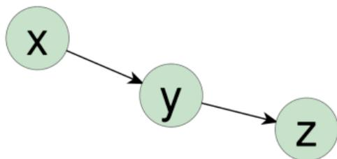
$$p(x, y, z) = p(x | y)p(y | z)p(z) = p(z | y)p(y | x)p(x)$$
