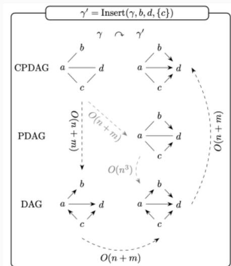
Linear-time approach for applying a GES operator.
