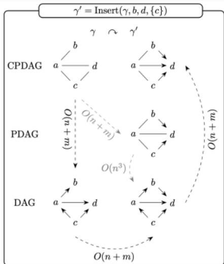
Linear-time approach for applying a GES operator.
