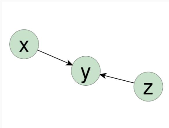
A **DAG** is a directed graph such that following arrows it is impossible to return to any vertex (no cycles). A **PDAG** has additional undirected edges.
